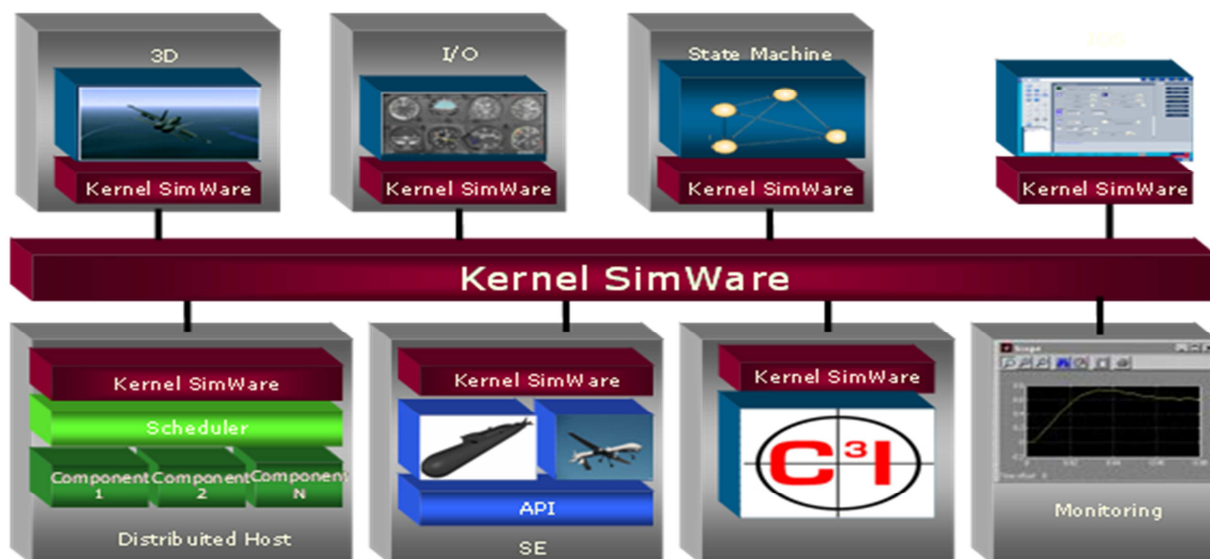
Fig. 2. Esquema general del framework SimWare, de Nextel Engineering Systems S. L.
